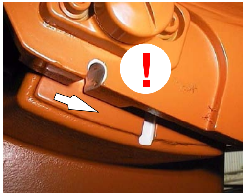
Pre-mastering position of axis 3
