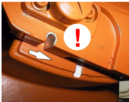
Pre-mastering position of axis 3
