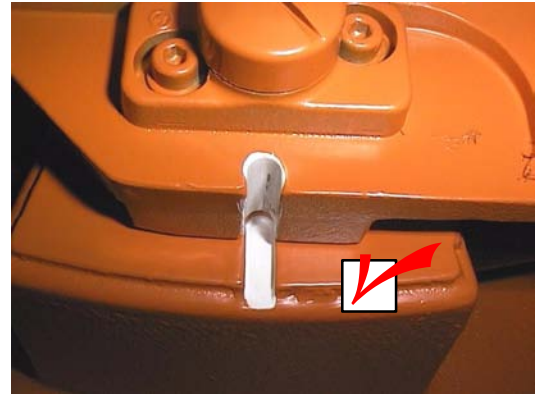
Pre-mastering position of axis 3
