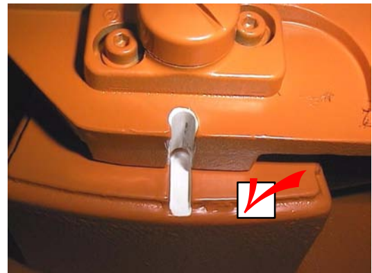
Pre-mastering position of axis 3
